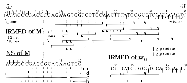
Figure 4. MS data providing sequence of 50-mer treated as an unknown (symbols as in Figure 2, and mass values in Table 2). Other internal ions for which multiple sequence assignments are possible are listed in the supporting information, Table 1. Asterisk: unique to 13 ms IRMPD. Dark (light) bars: mass error \leq \pm 0.05 Da, average \pm 0.02 ( \leq \pm 0.25 Da, average, \pm 0.12 ).
